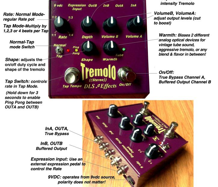
Warmth Pot: A first ever Warmth pot allows the user to dial in Vintage tube sounding tremolo to modern edgy tremolo, or any blend of the two sounds. This is achieved by biasing 2 different sounding analog optical-couplers via the Warmth pot.
