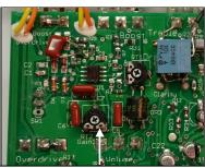
Stage 2 Drive pot: Factory Set to 50% rotation. CCW = more distortion edge CW= less distortion, clearer
