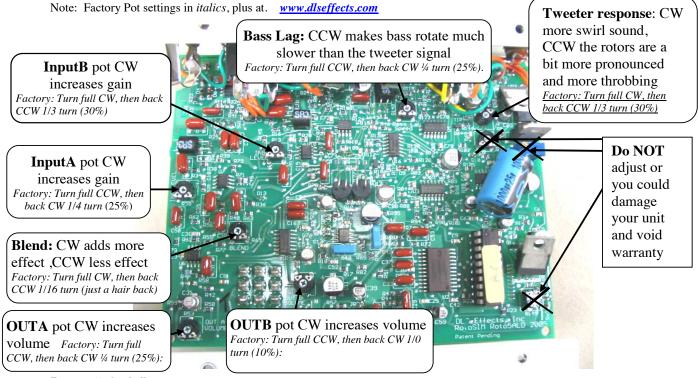
**Power "+9vdc":** Input for 9 to 13.8vdc, 90ma minimum, 2.1mm jack, <u>polarity does not matter</u>. (DC adapter included) **Note:** The RotoSIM requires a minimum of 9vdc to keep the effect depth at maximum. If in question, use the supplied transformer or higher voltage input within the range of 9vdc to 13.8vdc.
