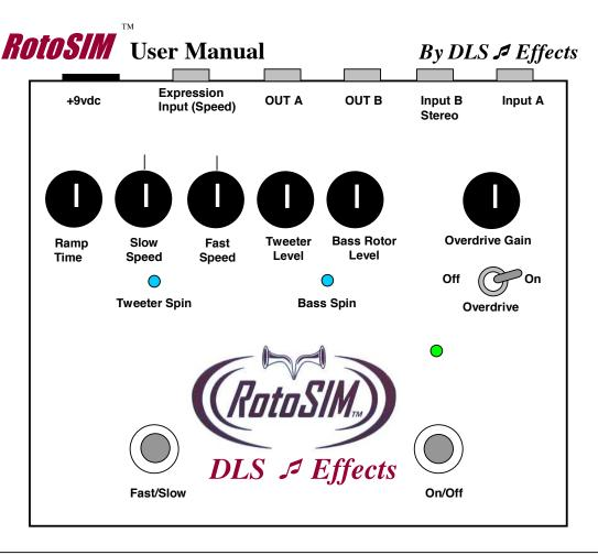
**Note1:** Output A is designed to sound slightly different than Output B. OUTA is a little more transparent and truer sounding. Output B is deeper and thicker sounding. The musician can experiment with both outputs while the instrument is plugged into INA. (This also gives a nicer stereo sound spread when used in stereo).
